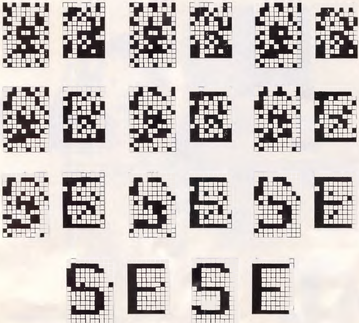
Fig 2 Asynchronous recall in a BAM consisting of two fields of neurons, one containing 140 neurons and another containing 3 neurons
